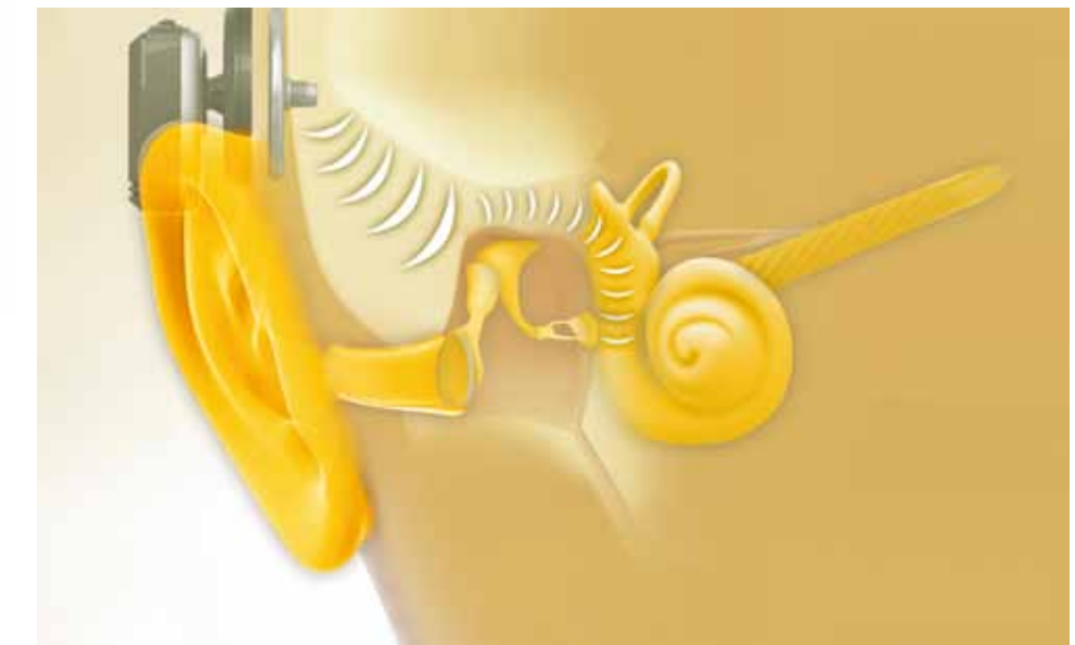
Figure 5. Bone conduction hearing implant – transcutaneous.
